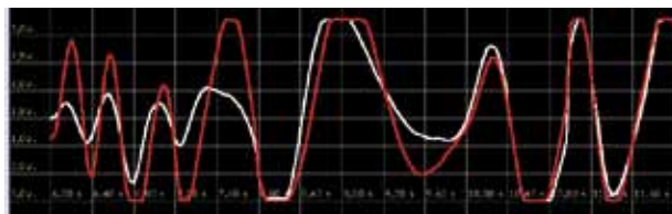
With active SCP function: the signals of the two PIR are homogenous; the alarm is triggered off
